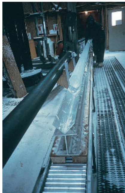
FIGURE 10-2 Ice coring operations (A, B) Ice drilling during cold “summer” conditions retrieves sequences of ice cores thousands of meters thick. (C) Scientists may also examine upper ice layers in pits dug into the ice. (Courtesy of Paul Mayewski, University of Maine.)
