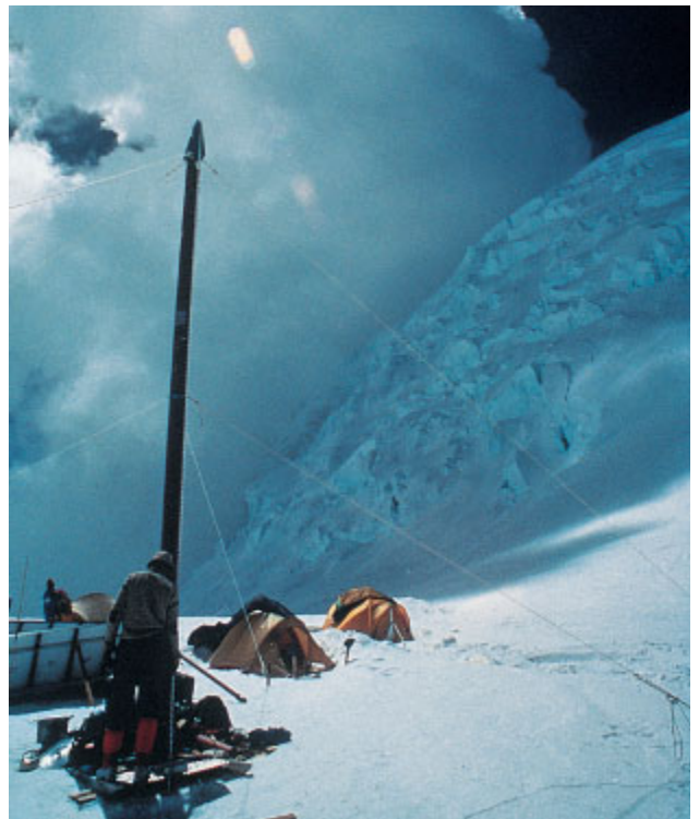
FIGURE 16-3 Coring mountain glaciers Drilling ice cores from (A) annually layered mountain ice requires (B) hauling equipment and supplies up and down the sides of mountains and ice caps and then (C) drilling at elevations approaching 20,000 feet, sometimes with (D) towering summer storm clouds rising from lower elevations and looming in the background. (Courtesy of L. G. Thompson, Byrd Polar Research Institute, Columbus, OH.)
