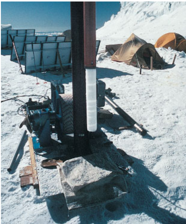
FIGURE 16-3 Coring mountain glaciers Drilling ice cores from (A) annually layered mountain ice requires (B) hauling equipment and supplies up and down the sides of mountains and ice caps and then (C) drilling at elevations approaching 20,000 feet, sometimes with (D) towering summer storm clouds rising from lower elevations and looming in the background. (Courtesy of L. G. Thompson, Byrd Polar Research Institute, Columbus, OH.)
