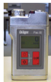
Electrochemical CO detector with direct measurement
