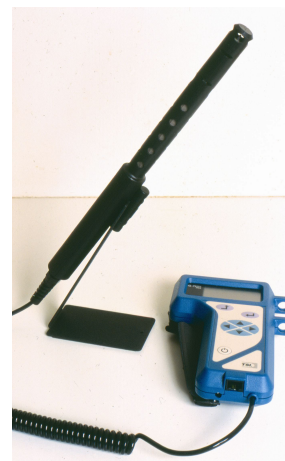
Temperature, relative humidity and carbon dioxide measurement instrument (Q-Track)
