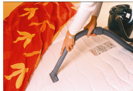
Data collection by suction of dust mites on a mattress
