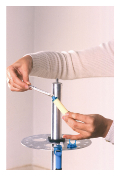
Solid adsorbent support used for data collection of VOC and aldehydes
