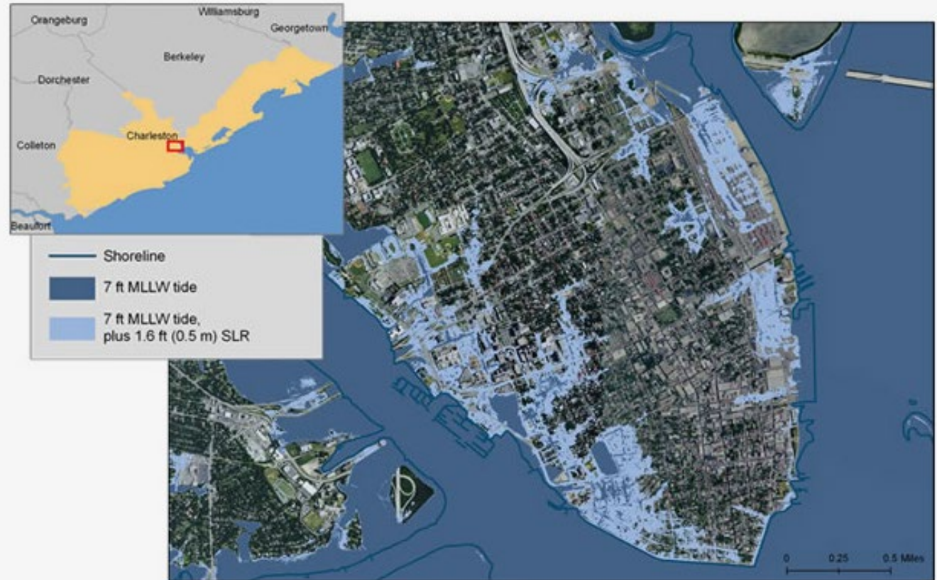
Example of potential inundation from coastal flooding, with and without sea level rise (SLR). (Does not account for erosion, subsidence, wind, rainfall, or future construction.)
