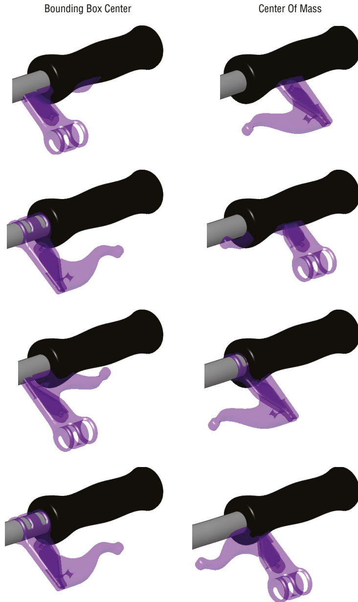
FIGURE 15.5 The mirror results of the Bounding Box Center and Center Of Mass options
