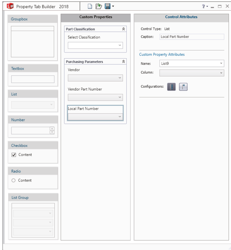
FIGURE 11.11 Using the Property Tab Builder to construct a Custom Properties tab for the Task pane
