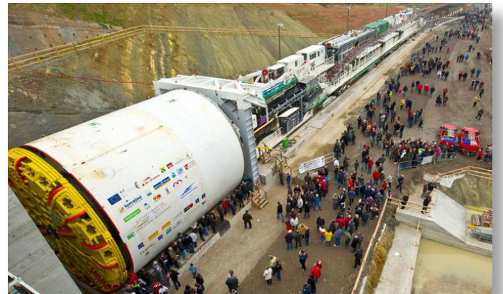
TBM Tunnel Boring Machine (max diam. 15 m)
