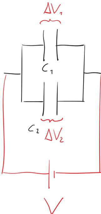
$$Q_T = Q_1 + Q_2 = C_1 V_1 + C_2 V_2 = V [C_1 + C_2]$$
