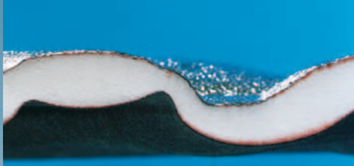
Shaped part with aluminum foil and felt
