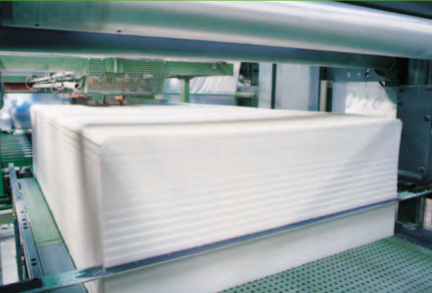
Cutting of Basotect® panels
