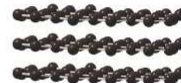
Graphite exists in planar sheets of benzene rings, held together by weak intermolecular forces.
