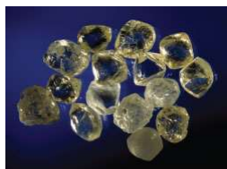
diamond an "infinite" array of six-membered rings, covalently bonded in three dimensions
