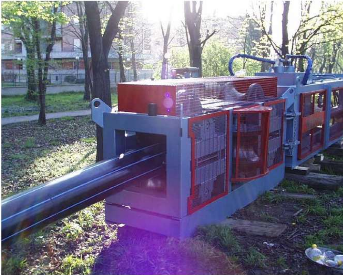
Roll-Down machine for longitudinal deformation of HDPE pipe to Pn16
