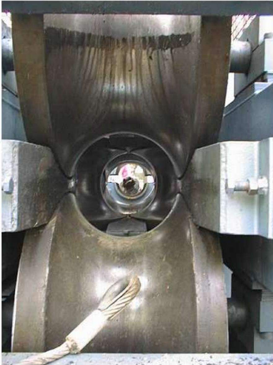
opposed rollers for reducing diameter and insertion of drawn pipe
