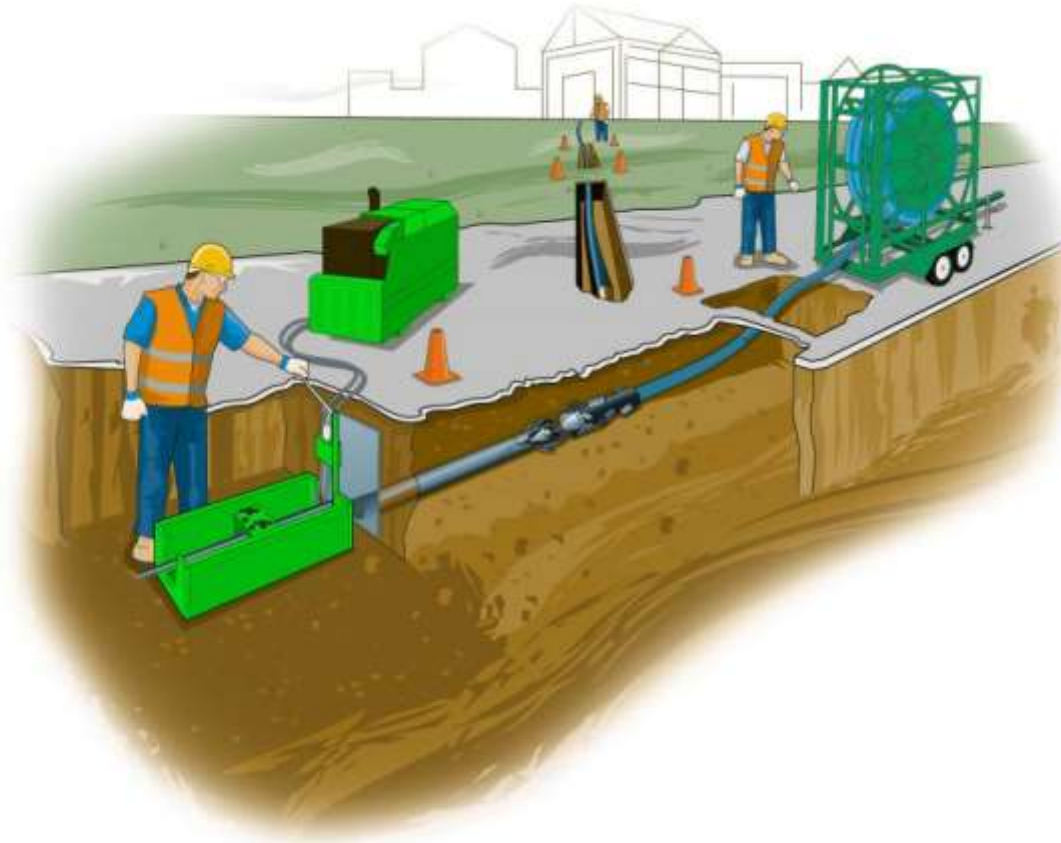
Typical small diameter static pipe bursting operation.
