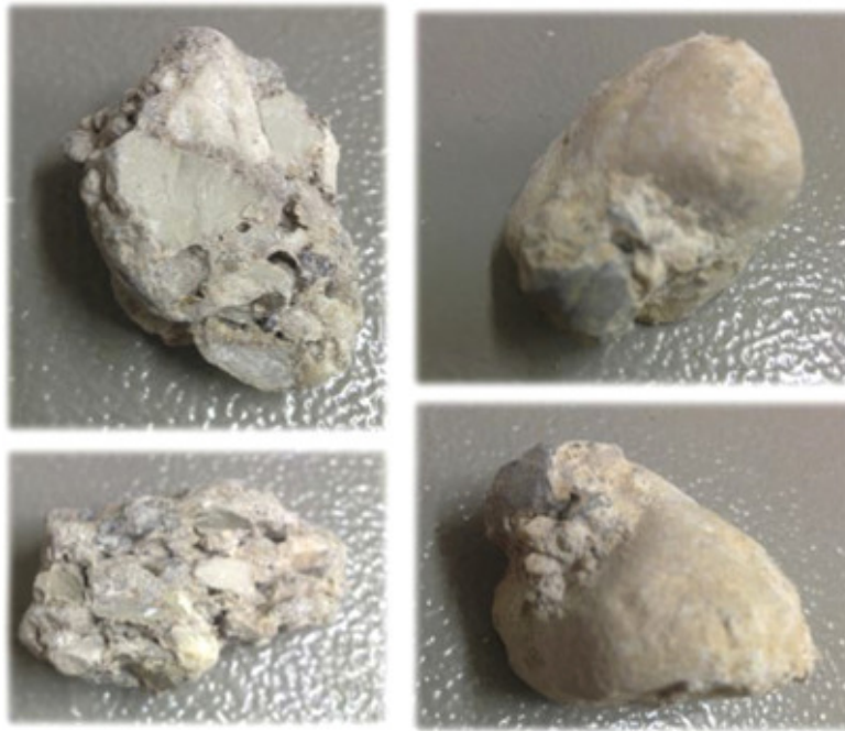
Figure 2.2. Recycled concrete aggregate (RCA) particles with different content of old attached mortar.
