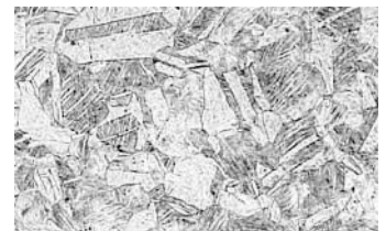
steel 1.4404 rolled solution annealed steel, and then drawn
