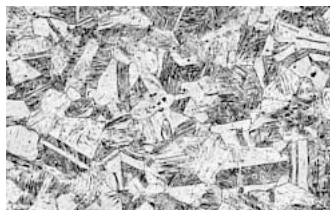
steel 1.4401 rolled solution annealed steel, and then drawn
