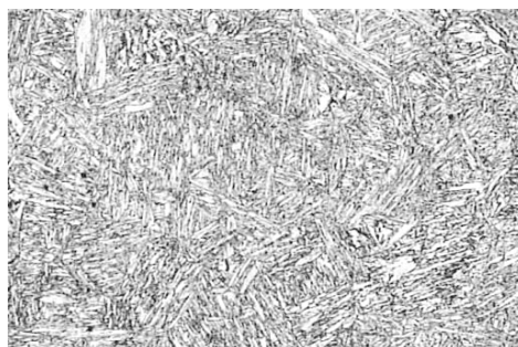
HARDENED STEEL 1.4006 X 200 tempered martensite
