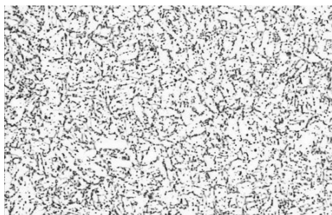
ANNEALED STEEL 1.4006 X 500 slight grain-boundary carbide precipitation
