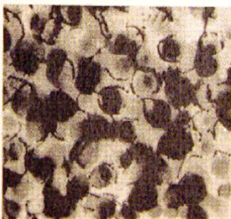
h. Dislocations Decorating \gamma' in U500 Tested at 1450F (790C). Transmission, 4,800X. Phillips 16
