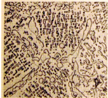
g. Condensed \gamma' in U700 Aged 180 Days at 1900F (1040C) 545X
