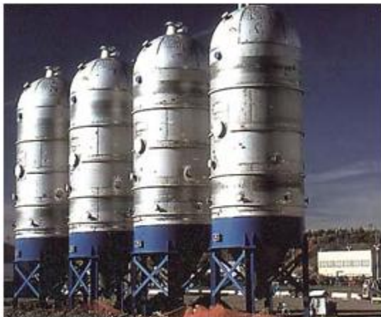
Figure 9. Pulp and paper 2205 digesters at Potlatch, USA manufactured with Industeel 2205 plates 3 .
