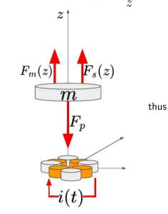
$F_m(z)\mapsto F_m\left(z_0\right)+\frac{\partial F_m\left(z_0\right)}{\partial z}\widetilde{z}$  s  $\frac{b_m}{z}\mapsto \frac{b_m}{z_0}-\frac{b_m}{z_0^2}\widetilde{z}$
