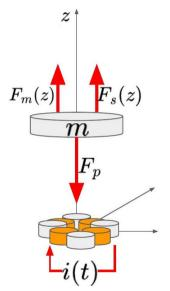
use simulink or numerically integrate the ODE
