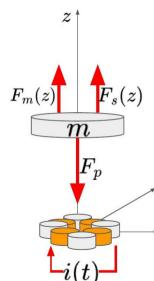
$$F_s(i,z) \mapsto F_s(i_0,z_0) + \frac{\partial F_s(i_0,z_0)}{\partial i}\widetilde{i} + \frac{\partial F_s(i_0,z_0)}{\partial z}\widetilde{z}$$
