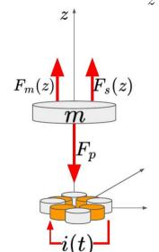
$$F_{m}(z) \mapsto F_{m}(z_{0}) + \frac{\partial F_{m}(z_{0})}{\partial z} \widetilde{z}$$
