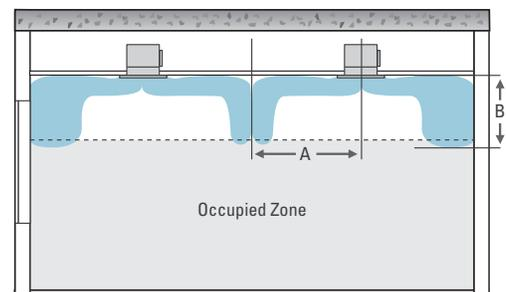
**Figure 25:** Ceiling diffuser free space mounting
