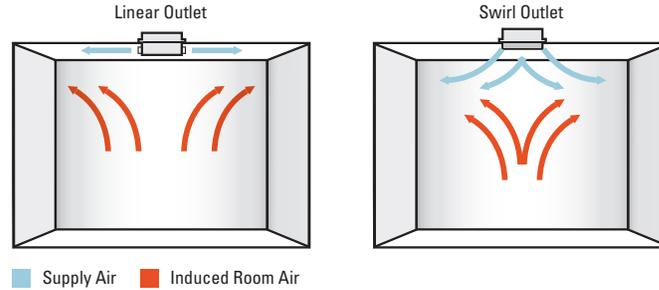
**Figure 35:** Variable volume supply with low temperature air outlets
