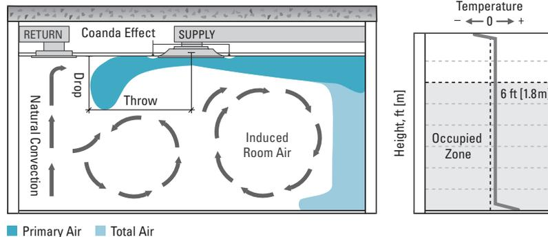
**Figure 2: Space air diffusion with overhead heating**
