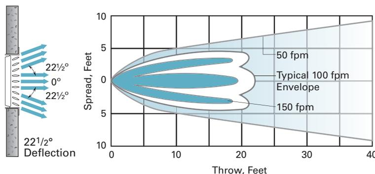
Handbook for a more detailed explanation. Good air distribution design makes use of room surfaces to help keep the supply air outside the occupied zone.
