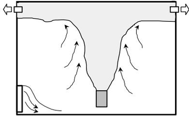
Also, a room with more stratification will reduce the relative density of the plume and, as a result, limit the height to which the plume will rise. The ceiling will stop the thermal plume. As a result there is an upper zone with high concentration of contaminants and high temperatures. The occupant zone will present lower pollutants concentration.
