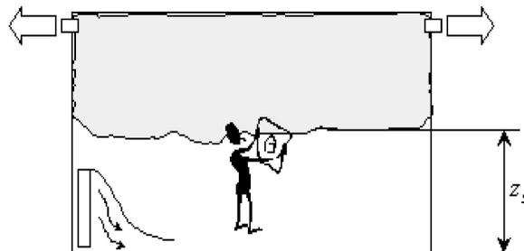
The displacement ventilation system is suited for ventilation and cooling systems. The system is not suited for heating. In case of heating an additional water based system with low room air velocity is needed (radiant panels or even radiators).
