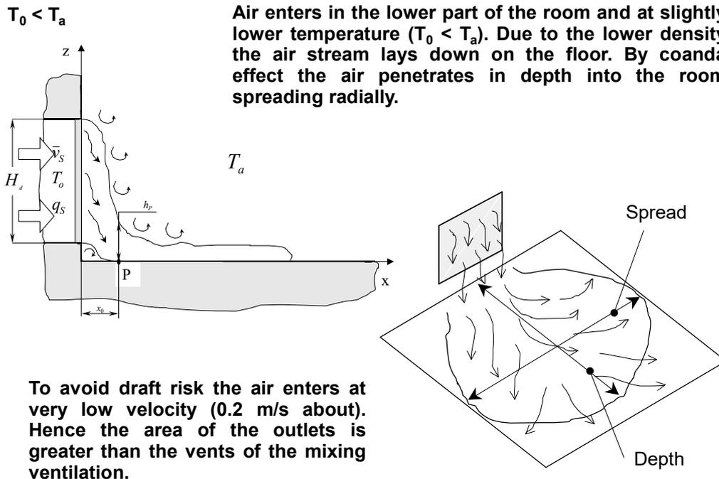
**Mechanism 2: thermal plume**
