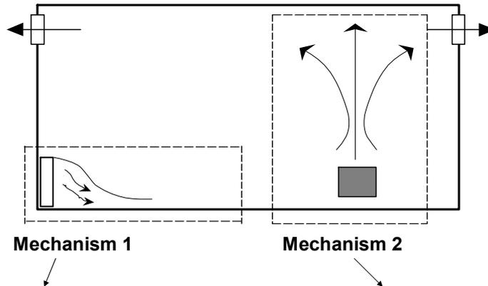
Air is introduced into the space at low velocities, which causes minimal induction and mixing. Displacement outlets may be located almost anywhere within the room, but have been traditionally located at or near floor level.
