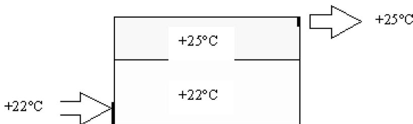
With the displacement principle heat and pollution is transferred from the residence zone close to the floor - to the ceiling where it is evacuated through the outlet system.
