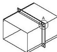
Slide-on cleats to press the flanges (bolt holes in the corners)
