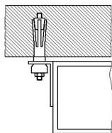
Suspended rectangular duct with expansion plug
