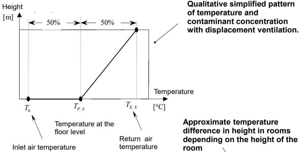
The temperature difference between ankle and head (0.1 m – 1.1 m) for seated sedentary persons has to be considered as local discomfort parameter. With higher activity and standing person, less problems.
