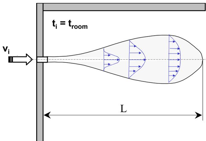
The **AIR THROW** is defined as the distance along the jet axis from the inlet to the section where the velocity has diminished down to the limit velocity  $v_{lim}$ . Usually this value is supposed to avoid local discomfort (DR) and hence the  $v_{lim} = 0.15 \div 0.25$  m/s in the occupied zone.
