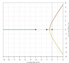
... while the poles of a system are very important in determining the behavior of a system, the zeros can also be important. After performing a root-locus design, it is critical to go back and test the closed loop system to ensure that it behaves as expected.
