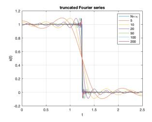
2. This exercise repeats the previous one in its first part, then re-evaluates the coefficients by numerical integration trough a cycle on M where samples nT and s(nT) are first stored, then used for calculating the approximate coefficients through a sum. The plot is zooming on the signal part that better evidences details, to appreciate how only M = 1000 is able to closely match the true result.
