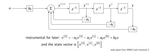
This shows how to rearrange a higher-order differential equation into a form suitable for state-space representation.
