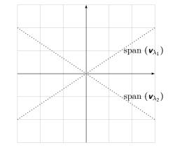
the trajectory along each eigenspace is driven by a first order differential equation  $\implies$  if  $\mathbf{x}_0 \in \operatorname{span}(\mathbf{v}_{\lambda})$ , then  $\mathbf{x}(t) = e^{\lambda t} \mathbf{x}_0$
