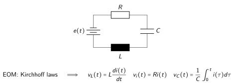
$$e(t) = v_L(t) + v_R(t) + v_C(t) \implies e(t) = L \frac{di(t)}{dt} + Ri(t) + \frac{1}{C} \int_0^t i(\tau) d\tau \quad (4)$$
