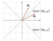
$\begin{array}{l} \textit{eigenspaces} = \textit{subspaces spanned by the eigenvectors} \\ \begin{bmatrix} 2 & 1 \\ 1 & 2 \end{bmatrix} \begin{bmatrix} x_1 \\ x_2 \end{bmatrix} = \lambda \begin{bmatrix} x_1 \\ x_2 \end{bmatrix} \quad \mapsto \quad \mathbf{v}_{\lambda=1} = \begin{bmatrix} 1 \\ -1 \end{bmatrix}, \quad \mathbf{v}_{\lambda=3} = \begin{bmatrix} 1 \\ 1 \end{bmatrix} \end{array}$
