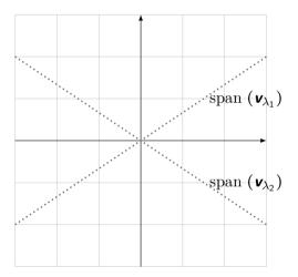
the trajectory along each eigenspace is driven by a first order differential equation  $\implies$  if  $\mathbf{x}_0 \in \operatorname{span}(\mathbf{v}_\lambda)$ , then  $\mathbf{x}(t) = e^{\lambda t} \mathbf{x}_0$
