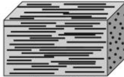
Aligned direction Fiber composite
