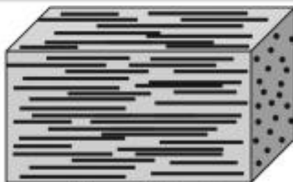
Aligned direction Fiber composite
