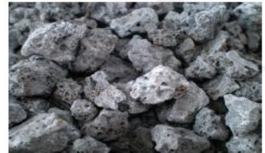
Electric Arc Furnace Slag (EAFS)
