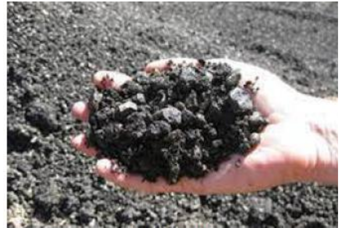
Reclaimed Asphalt Pavement
