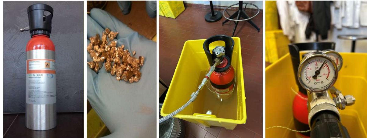
From left to right: MyH2_3000; metal hydride powders; charging process; discharging process
