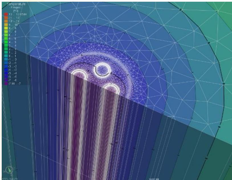
Freeze-thaw cycles induced in cohesive sediments around the BHE → deformations of the ground level + change in the permeability + alteration of the thermal exchange and energetic performances
