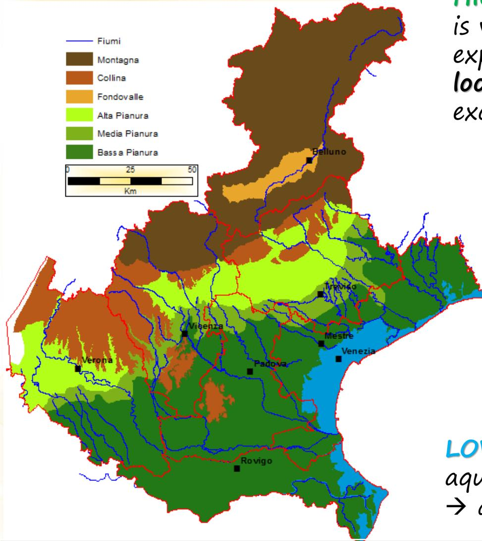
**HIGH PLAIN AREAS:** the water table is very low → open loop systems are expensive and not effective / **closed loop** are highly efficient, high thermal exchange due to high groundwaterflow
