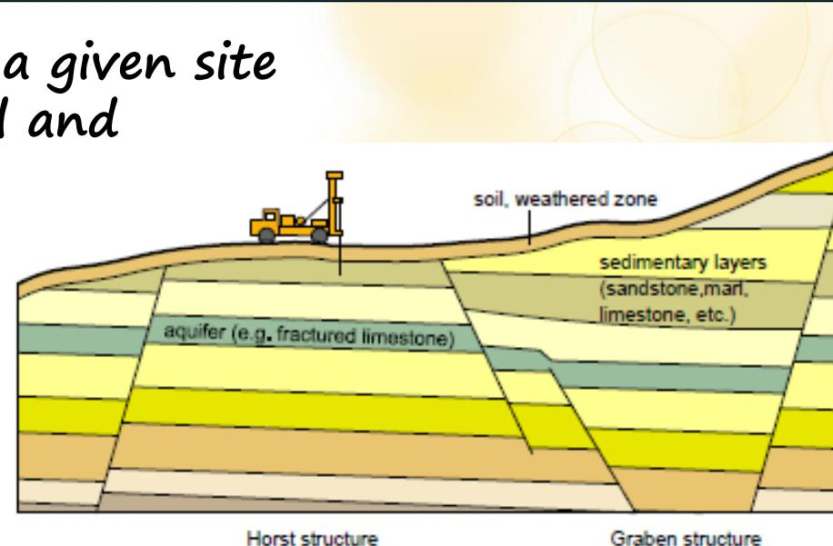
2) Mesozoic sediments resting sub-horizontal or tilted, often intersected by faults.
