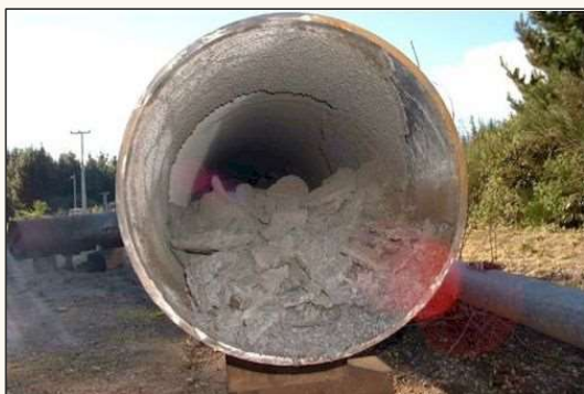
Silica deposit in geothermal fluid line (left) and steam turbine (below left / right)
