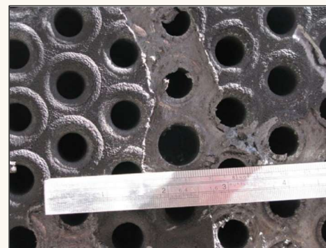
Antimony sulphide deposition on a heat exchanger from a geothermal (binary) power plant.
