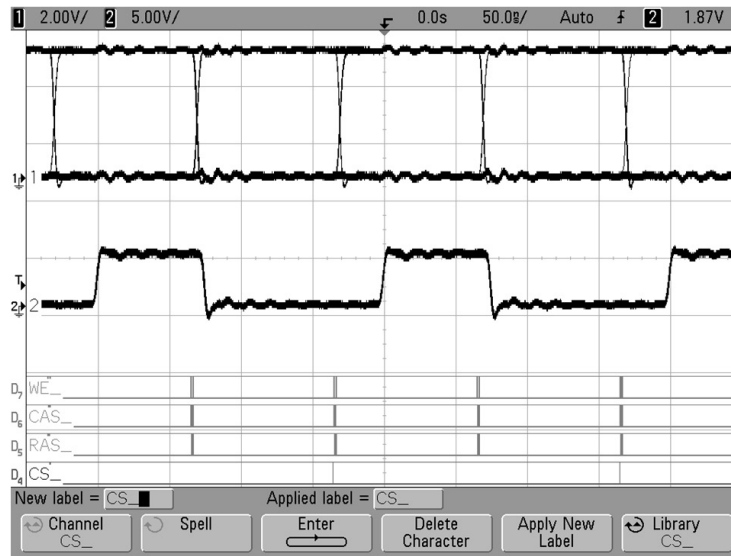
Figure 1.1: Label menu softkeys are shown in the lower part of the screen.
