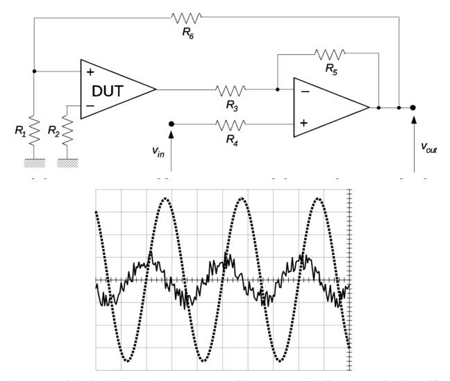
The purpose of the circuit is to enable measurement of the open-loop gain for the operational amplifier indicated as DUT. Waveforms measured at the test circuit input and output are represented by the two oscilloscope traces shown in the figure that follows, respectively:
