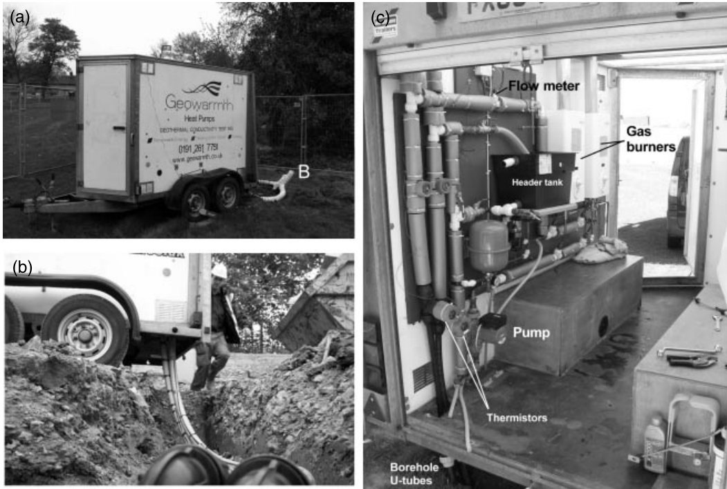
Figure 15.6 (a) A self-contained trailer-mounted test rig operated by Geowarmth Heat Pumps Ltd. and powered by liquid petroleum gas ( photo reproduced by kind permission of Geowarmth Heat Pumps Ltd. ). The borehole head is marked by 'B'. (b) The ground loop running from a test borehole at the Annfield Plain site (Box 11.2) to the test rig ( reproduced by kind permission of Pablo Fernández Alonso ); (c) the interior of the test rig ( photo by David Banks ).
