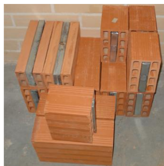
Figure 12. Clay bricks including PCM macro-capsules [61].
