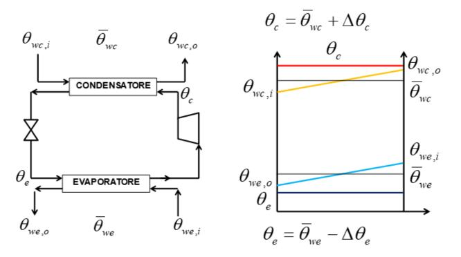
Condensing heat released to water fluid
