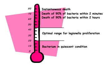
**Indirect systems** limit the water stagnation. **Direct systems:** usually there is the need of thermal cycles (above 60°C) to prevent the problem (usually one night per week with an electric resistance)
