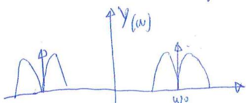
$$Y(\omega) = A \pi \delta(\omega - \omega_0) + \frac{1}{2} \frac{A}{X_{\max}} X(\omega - \omega_0)$$
