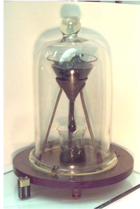
Pitch drop experiment apparatus
