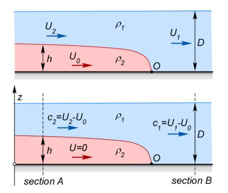
To analyze how front moves forward, it is appropriate changing the reference system with the one centered in O translating with  $U_0$ , that is the velocity of the toe. The new scheme of the problem is reported in the present picture.
