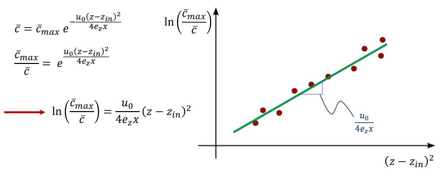
**N.B.** The goodness of fitted data depends mainly of the position of  $z_{in}$ . When  $z_{in}$  is close to  $z = z_0$ , 0 we can have significant error in the estimation of  $e_z$  ( $\varepsilon > 10 \div 20\%$ ).
