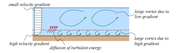
The vortexes within the boundary layer have <u>higher intensity</u> and <u>stronger anisotropy</u> than the vortexes in the external region.
