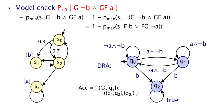
• Result:  $\underline{p}_{min}(G \neg b \land GF a) = [0, 0, 0, 1]$ - Sat(P<sub>>0</sub> [G  $\neg b \land GF a$ ]) = {s<sub>3</sub>}
