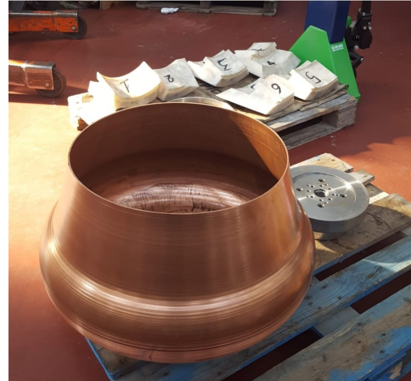
READY FOR THE SPINNING OF 2° HALF CELL
