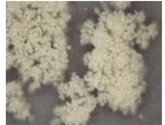
Sulfur removed from a PVDF tube
