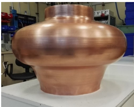
3rd Thermal Annealing
