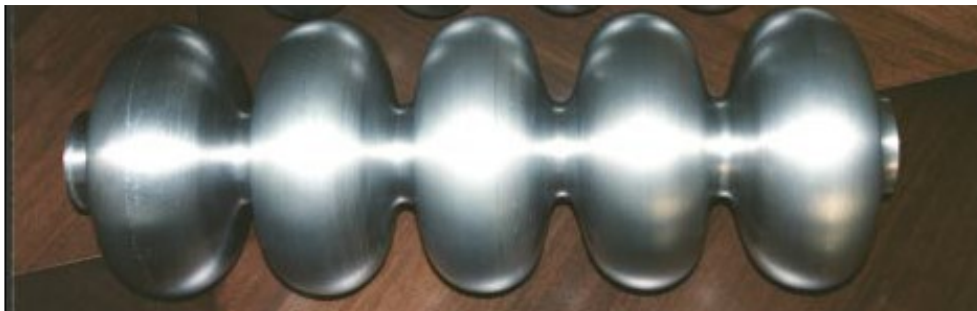
First seamless multicell by spinning
