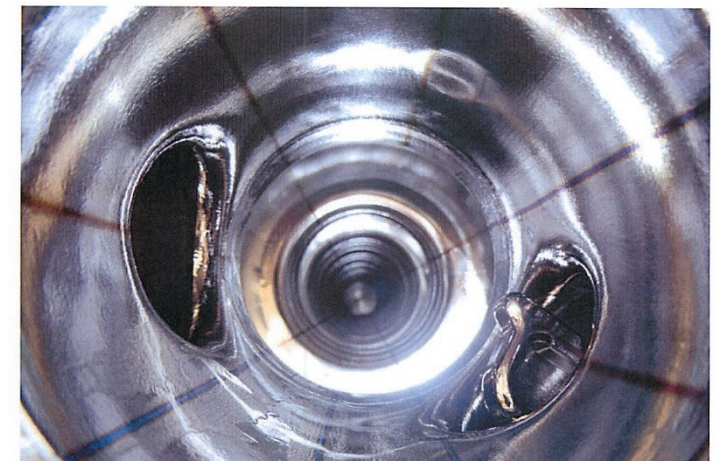
Oxidation induced by fixed HPR jets
