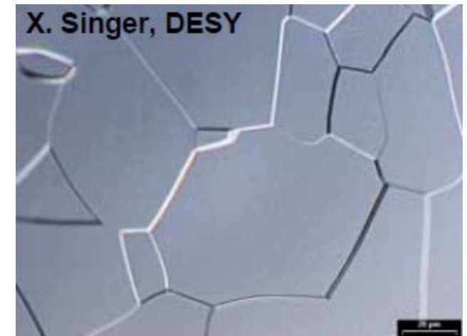
Completely recrystallized Nb
