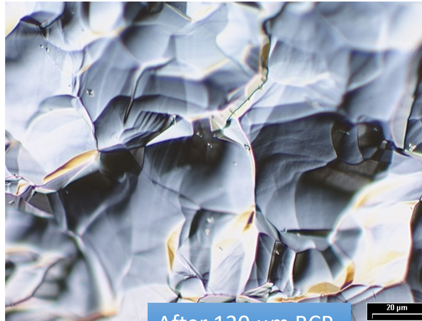
After 120 \mu\text{m} BCP
