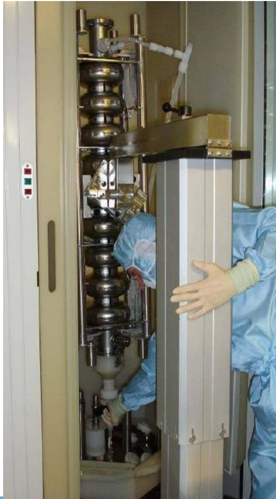
Rinsing cabinet of "old" DESY HPR system
