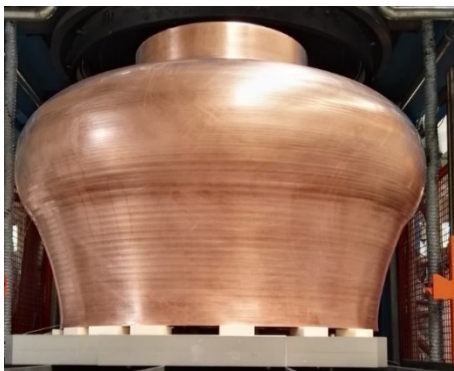
1st Thermal Annealing
