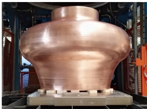
2nd Thermal Annealing
