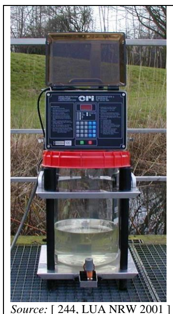
Figure 5.3: Example of an automated sampling device
