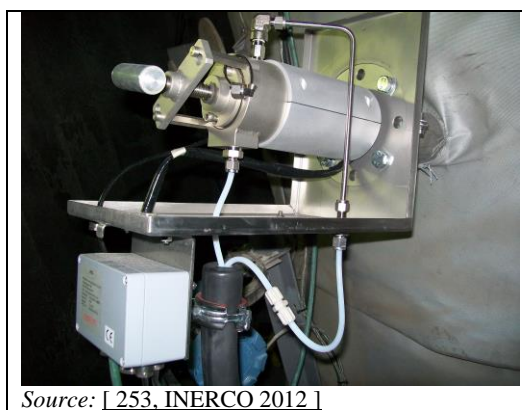
Figure 4.1: Example of an extractive sampling device
