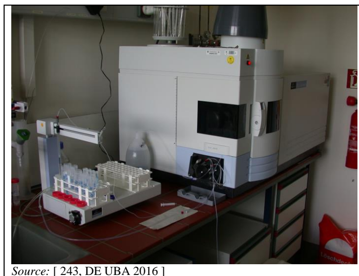
Figure 5.6: Example of an inductively coupled plasma optical emission spectrometer
