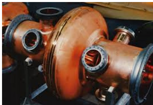
Elliptical 1 cells (LHC), protons and Pb, 400 MHz 5 MV/m, \beta = 1
