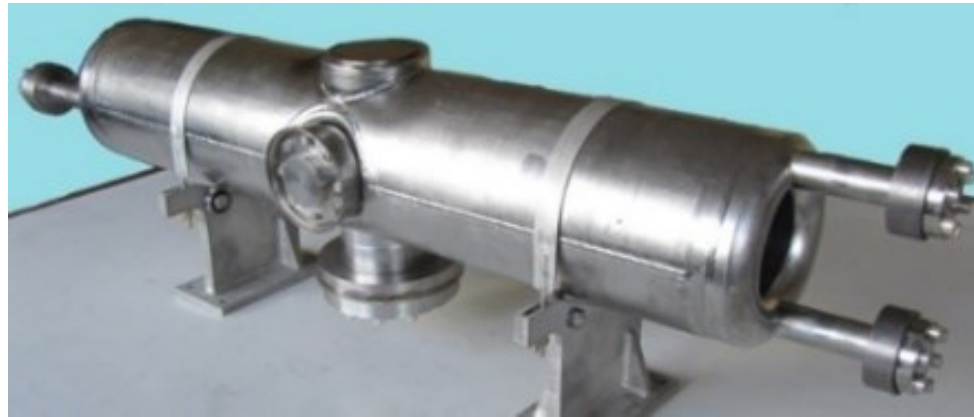
Half wave (IFMIF) deuterons, 175MHz, \beta = 0,092
