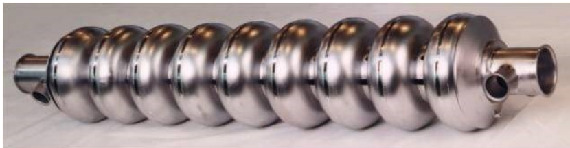
Elliptical 9 cells (XFEL - Tesla type ), electrons, 1.3 GHz 20-30 MV/m, \beta = 1
