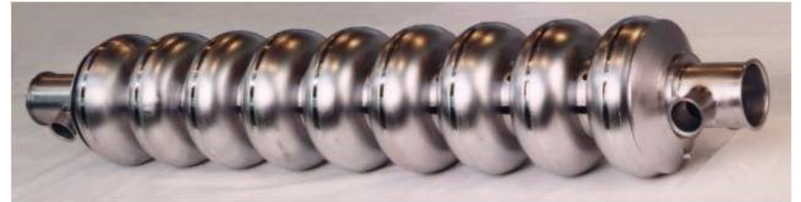
Elliptic 9 cells (XFEL - Tesla type ), electrons, 1.3 GHz 20-30 MV/m, \beta = 1
