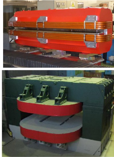
Dipoles to curve
