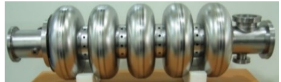
Elliptic 5 cells (ESS), protons, 704 MHz, \beta = 0,86
