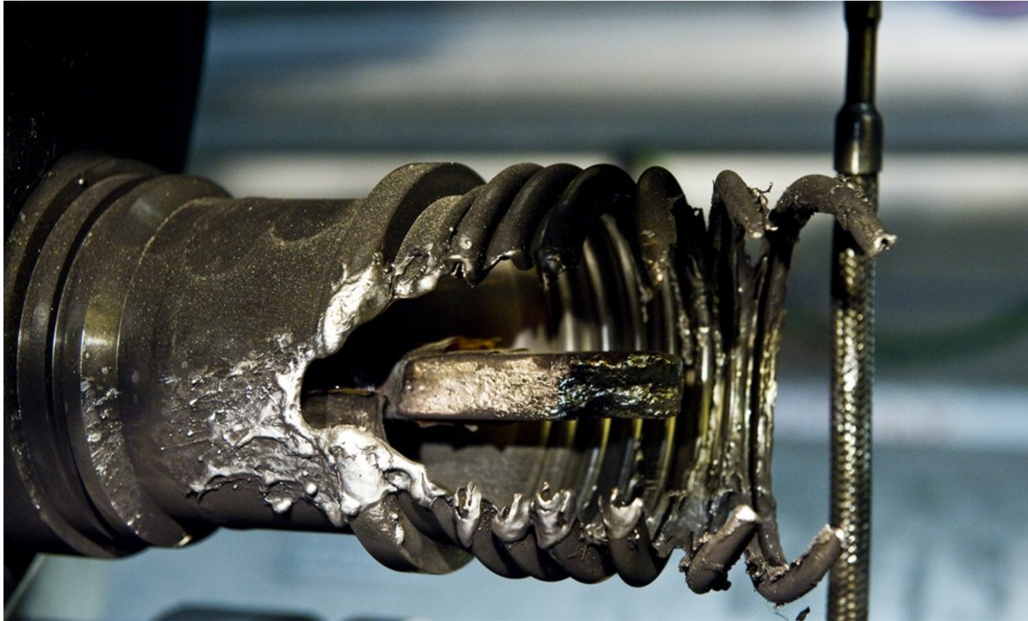
Detail of some of the damage done to the LHC magnets in sector 3-4 on September 19th, 2008. (Maximilien Brice, © CERN)
