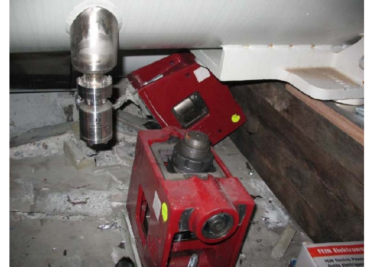
Obvious damage to concrete, where a magnet has been lifted off its mount (the red boxes) that secured it to the floor (CERN)
