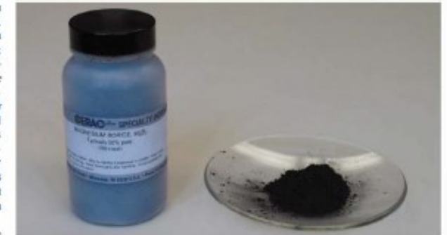
Figure 1 The newly discovered superconductor magnesium boride has been available in large quantities from suppliers of inorganic chemicals for many years, but physicists have finally 'rubbed the lamp' and found that magnesium boride superconducts at an amazing 39 K (ref. 1).
