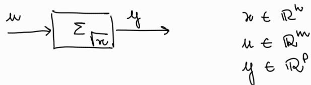
$$\begin{aligned} x(t) &= F x(t) + G u(t) & F \in \mathbb{R}^{n \times n} & H \in \mathbb{R}^{p \times n} \\ y(t) &= H x(t) + J u(t) & G \in \mathbb{R}^{n \times m} & J \in \mathbb{R}^{p \times m} \end{aligned}$$
