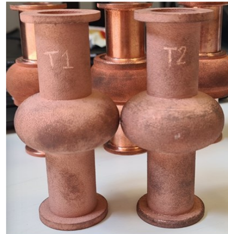
2 prototypes produced using TRUMPF TruPrint 5000
