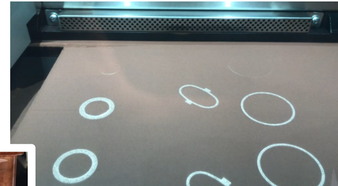
6 GHz seamless copper cavities via Additive Manufacturing
