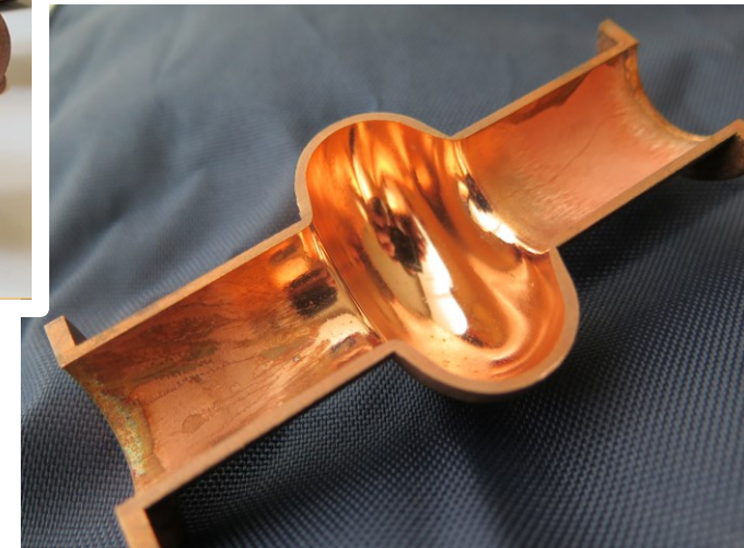
AM Cavity cutted after VB + EP of the cell
