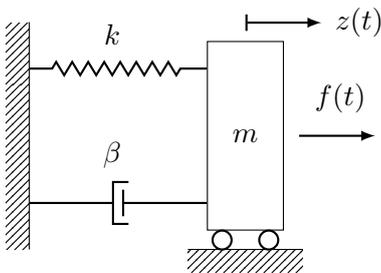
$f(t) = \text{input}, z(t) = \text{output}$
