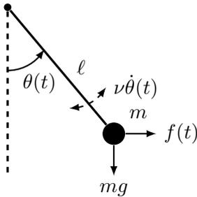
$f(t) = \text{input}, \theta(t) = \text{output}$
