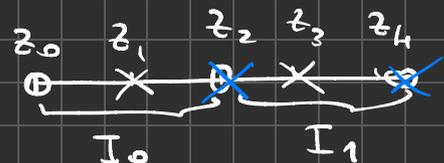
$$\int_a^b f(x) dx \approx \frac{h}{3} \left[ \underset{\parallel}{f(z_0)} + \underline{4} \underset{\parallel}{f(z_1)} + \underline{2} \underset{\parallel}{f(z_2)} + 4 \underset{\parallel}{f(z_3)} + \dots + 4 \underset{\parallel}{f(z_{2N-1})} + \underset{\parallel}{f(z_{2N})} \right]$$
