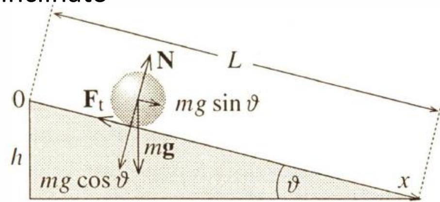
$$v_{Cf} = \sqrt{\frac{2gh}{1 + I_C/mR^2}} = \sqrt{\frac{2gh}{1 + (q/R)^2}} \quad \frac{U_{k,rot}}{U_{k,trasl}} = \frac{\frac{1}{2}I_C\omega^2}{\frac{1}{2}mv_C^2} = (q/R)^2$$
