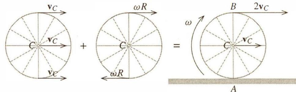
$$U_k = \frac{1}{2} m v_C^2 + \frac{1}{2} I_C \omega^2 = \frac{1}{2} m R^2 \omega^2 + \frac{1}{2} I_C \omega^2$$
