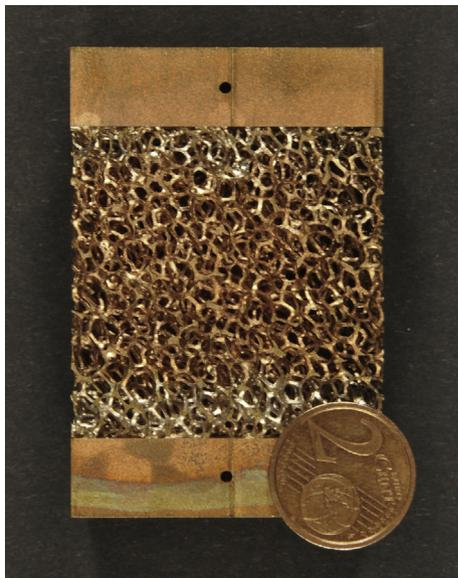
Fig. 2. Photo of a 10 PPI copper foam sample.
